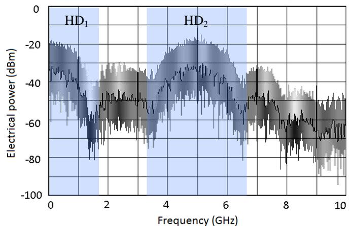
Figure 2 Transmitted electrical spectrum with HD<sub>1</sub> and HD<sub>2</sub> channels.
