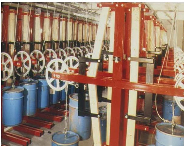
**Fig. 1** Long-term test rigs to accommodate two boards each
