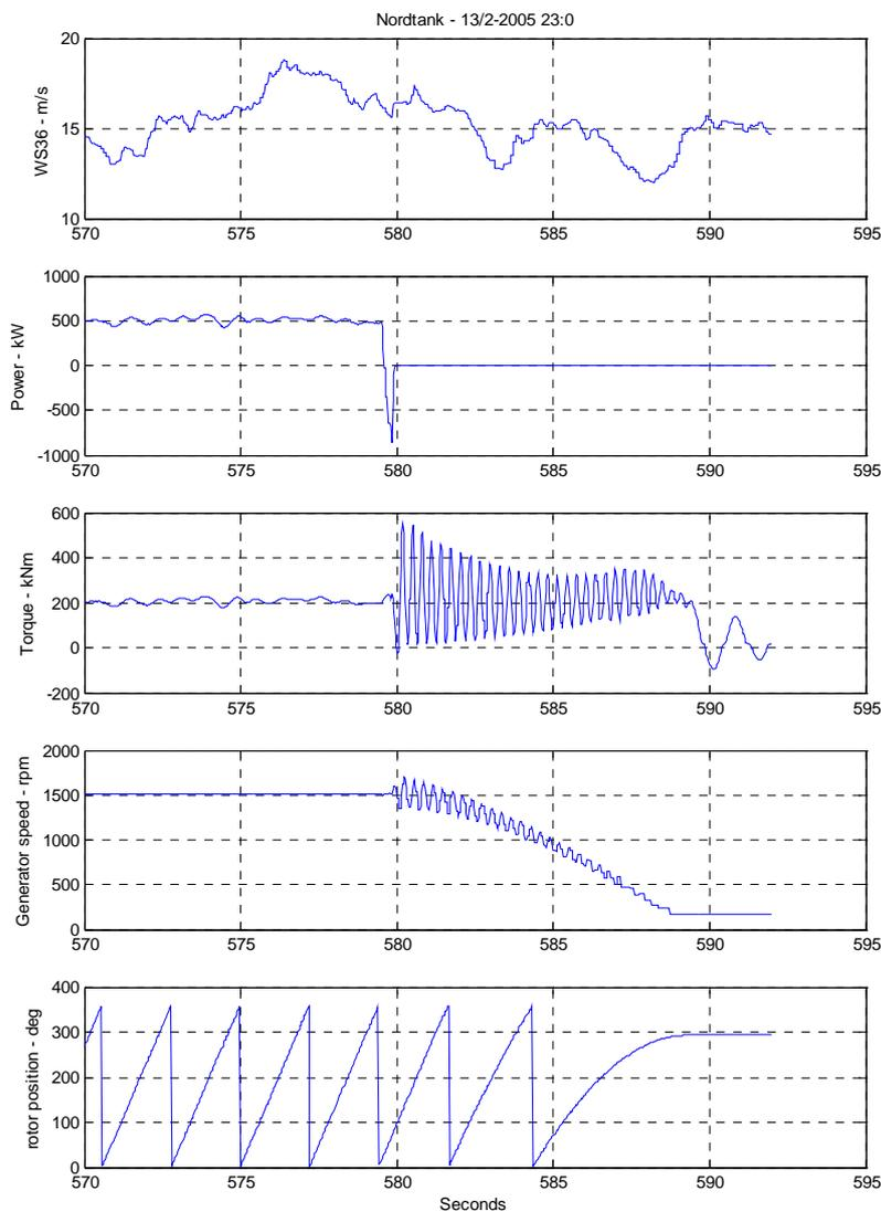
Figure 8: Example of recorded emergency stop.
