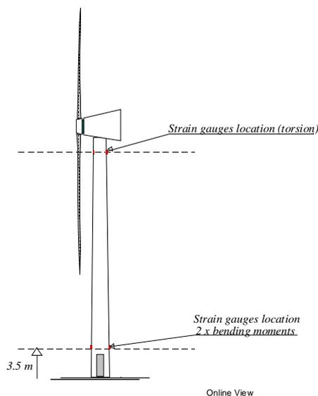
Figure 4: Structural load measurements in the tower of NTK 500/41 wind turbine.
