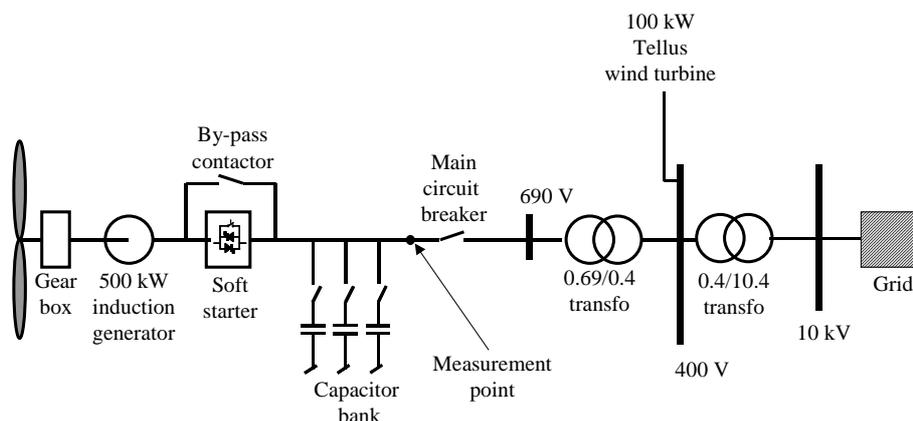
Figure 1: Connection diagram for NTK 500/41 wind turbine.
