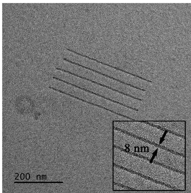
**Fig. 2** Patterned undecane ( $C_{11}H_{24}$ ) lines with average line widths of  $8 \pm 1$  nm. Patterning was carried out in an environmental transmission electron microscope operated at 80 kV in scanning mode with an estimated beam diameter of  $\sim 1$  nm and a beam current of  $\sim 0.53$  pA.
