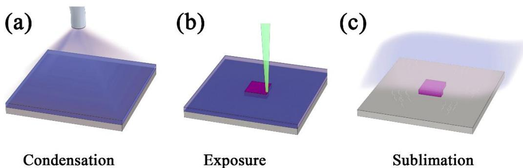
**Fig. 1** Organic ice resist patterning. (a) A vapor of organic precursor condenses on a substrate cooled down to cryogenic temperature. (b) During e-beam exposure, the chemical structure of the exposed area is altered resulting in the formation of a non-volatile product. (c) After heating the substrate to a room temperature, the unexposed resist sublimates, while the exposed area remains.
