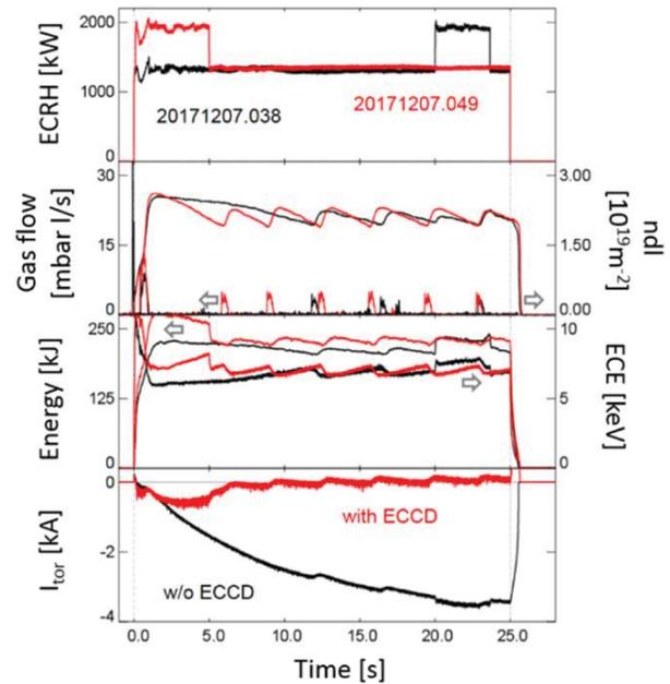
**Figure 5.** Comparison of two plasmas without (20171207.038) and with ECCD (20171207.049) to compensate the bootstrap current. The time traces (of ECRH power, gas flow and line integrated density, plasma energy, central electron temperature from ECE and plasma current) of the reference case without ECCD are plotted in black. In the counter-ECCD case (plotted in red), the total current (measured by a Rogowski coil) remains close to zero.
