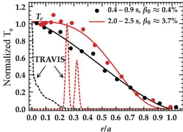
**Figure 4.** Shown are the normalized electron temperature profiles (from Thomson scattering measurements) for a plasma (#20171207.006) in which the central  $\beta$  increased from 0.4% (black) to 3.7% (red). The TRAVIS calculations (dashed curves) illustrate how the diamagnetic effect and the Shafranov-shift affect the ECRH power deposition profiles.
