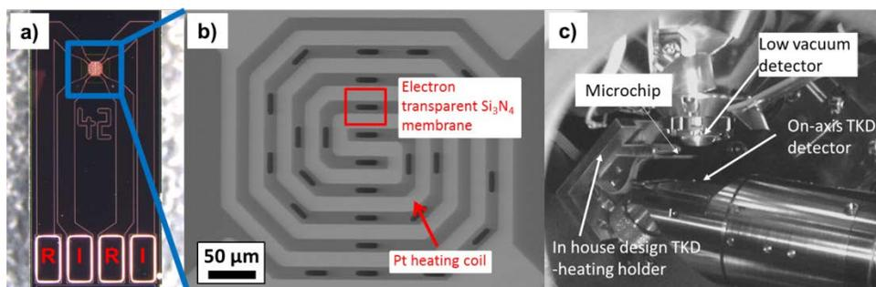
**Figure 1.** a) Structure of the MEMS microchip with resistance (R) and current (I) contacts highlighted. b) Zoom of the research area: the electron transparent Si<sub>3</sub>N<sub>4</sub> membranes and the embedded Pt heating coils are visible. c) Image of the TKD system configuration. The 45° tilted holder supporting the microchip and the on-axis TKD detector are visible.
