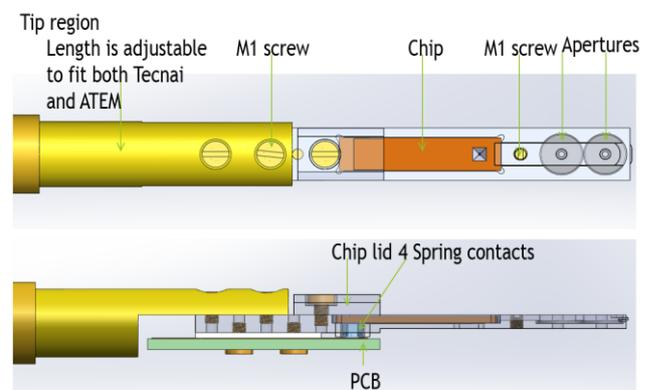
Figure 2: Schematic illustration of the electron biprism rod.
