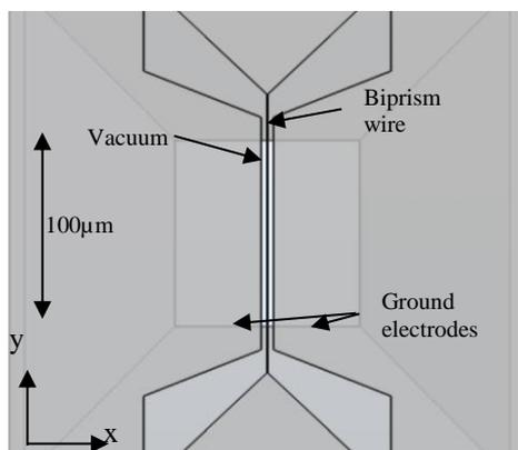
Figure 1: Design of the electron biprism chip.
