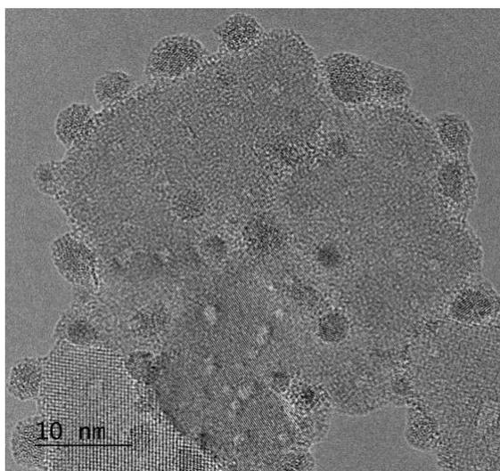
Figure 1: Rh particles on a TiO<sub>2</sub> support in 3 mbar H<sub>2</sub> illustrating the SMSI effect.
