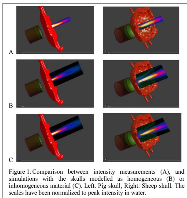
Figure 1. Comparison between intensity measurements (A), and simulations with the skulls modelled as homogeneous (B) or inhomogeneous material (C). Left: Pig skull; Right: Sheep skull. The scales have been normalized to peak intensity in water.
