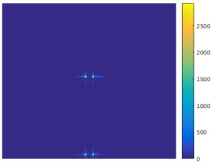
Figure 4. Measured as Fig. 3, but with the transmitter turned on with no modulation. The transmitter output power is  $-25.7\text{dBm}$  equal to  $2.7\mu\text{W}$ . The image is normalized, and the peak SNR is approximately 2000.
