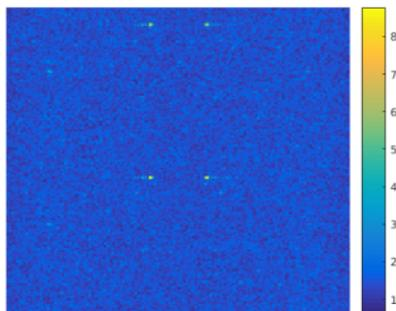
Figure 3. Measured noise MR image, acquired with the transmitter turned off, and the receiver adjusted to 120MHz. Weak irrelevant noise sources appear as dots in a thermal noise background.
