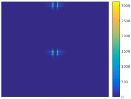
Figure 5. Measured as Fig. 4 but with additional  $3\text{V}_{\text{peak}}$   $10\text{Hz}$  sine wave AM. The transmitter output power is  $-25.7\text{dBm}$  equal to  $2.7\mu\text{W}$ .
