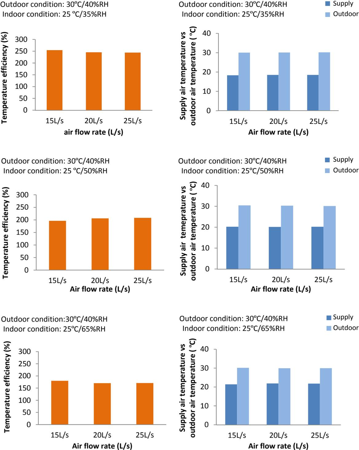
Figure 3. The measured temperature efficiencies and temperatures of supply and outdoor air at the three levels of airflow rate. The experiment was conducted at the simulated extreme Copenhagen summer climate and three air-conditioned indoor climate.
