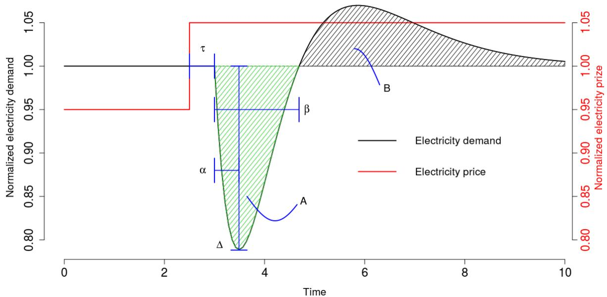
Figure 1 Example of response of a building's electricity demand to a penalty signal, where  $\tau$  is the time from the signal is submitted to an action starts,  $\alpha$  is the period from start of the response to the max response,  $\Delta$  is the maximum response,  $\beta$  is the duration of the response, A is the shifted amount of energy, B is the rebound effect for returning the situation back to "reference" [12].
