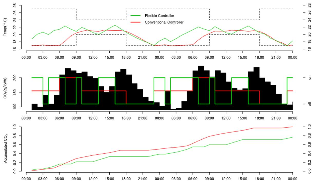
**Figure 2** Example of temperature control using two different controllers. In green is represented the flexible controller and in red the conventional one. In the top figure, the dotted lines represent the boundaries of the comfort conditions. The middle figure, the black rectangles represent the penalty signal, while in the bottom figure is represented the cumulative CO<sub>2</sub> emissions. (Source: DTU Compute)
