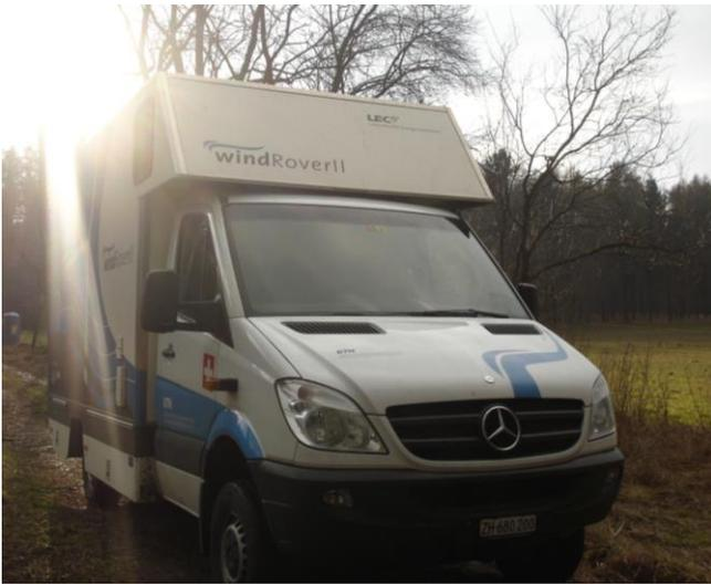
Fig. 1 Photograph of the mobile laboratory windRoverII that is equipped with the scanning LiDAR system. The LiDAR system is deployed through the roof of windRoverII.
