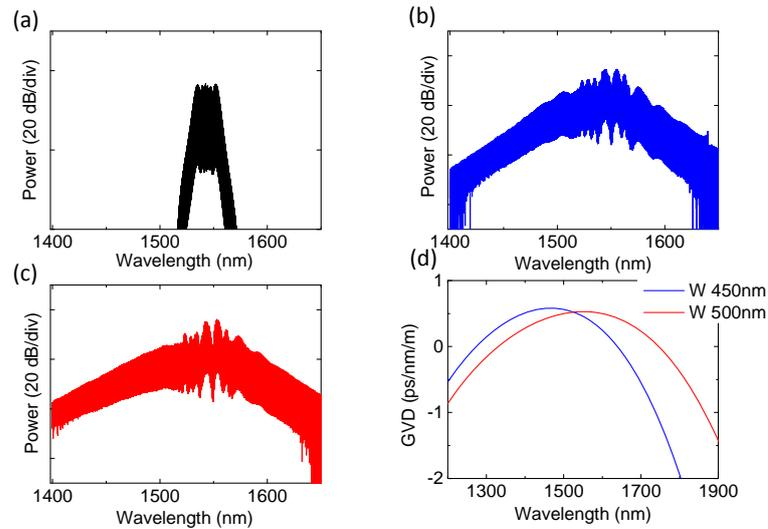
Fig. 2. Measured optical spectra at the input (a) and output of the AlGaAsOI nano-waveguide with the height of 290 nm and width of 450 nm (b) and 500 nm (c); the calculated group velocity dispersion (GVD) for the height of 290 nm and widths of 450 nm and 500 nm.
