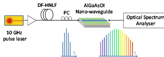
Fig.1 Experimental setup for spectral broadening in an AlGaAsOI nano-waveguide with a cross-section of 290×450 (or 500) nm<sup>2</sup>.
