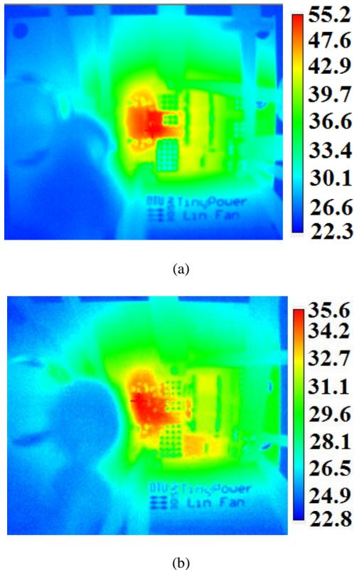
Fig. 11. Thermal images ( $^{\circ}\text{C}$ ) measured after one hour full-power operation, no heatsink, no airflow (annotated with output power, input voltage, nominal capacitance of C2, and switching frequency). (a) 10 W, 374 V, 3  $\mu\text{F}$ , 4 kHz. (b) 10 W, 300 V, 9  $\mu\text{F}$ , 1.5 kHz.
