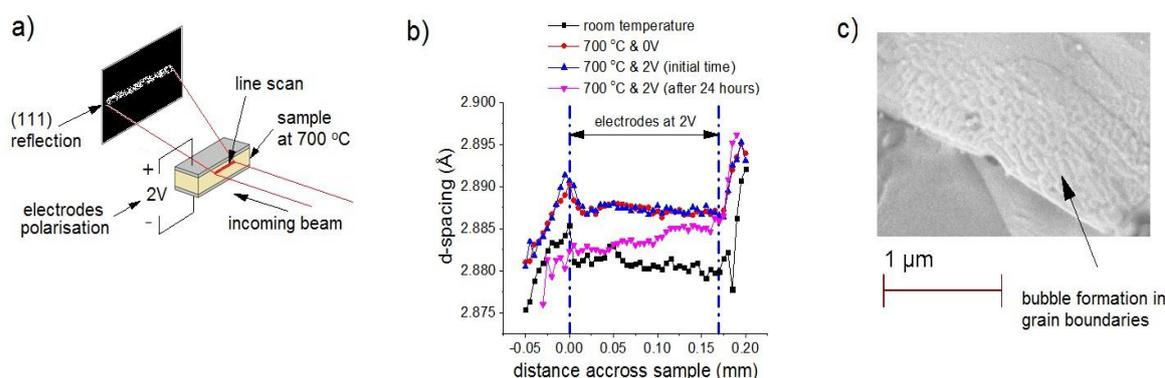
**Figure 1:** a) Scan position in the sample, parallel to the electrodes. b) Average position of peaks in each scan layer. c) Oxygen bubble formation in YSZ grain boundaries near oxygen electrode
