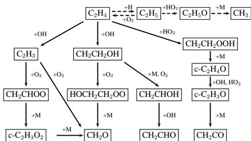
Figure 5: Main reaction pathways for  $C_2H_4$  conversion at the investigated conditions. The solid lines denote pathways important over the range of stoichiometries investigated, while dashed lines denote pathways important only under reducing conditions.
