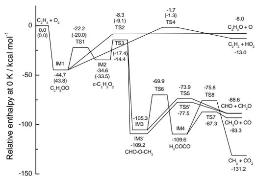
Figure 1: Relative enthalpies of minima and transition states for the  $C_2H_3 + O_2$  reaction computed at the CBS-QB3 level of theory. CCSD(T) results extrapolated to the complete basis set limit are shown in parentheses.
