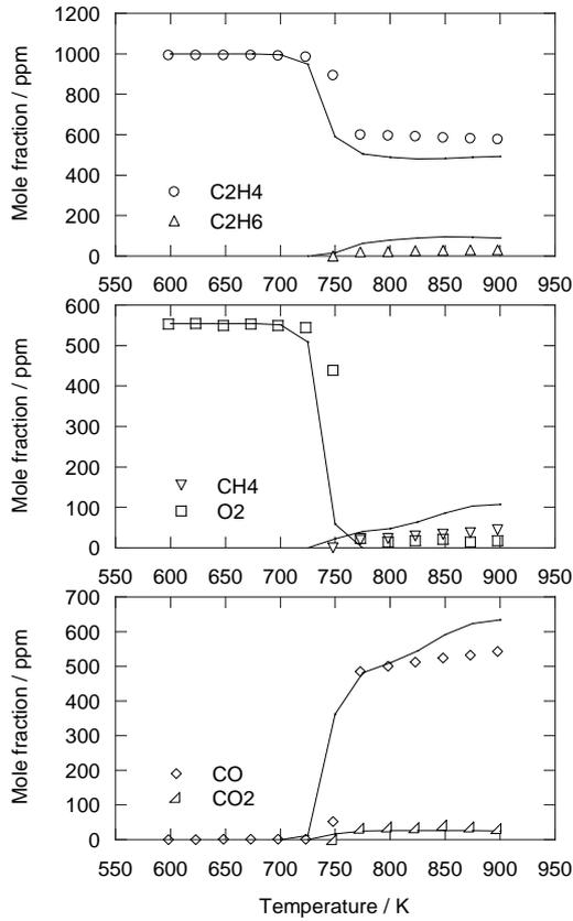
Figure 2: Comparison of experimental and predicted concentration profiles as a function of the reactor temperature for the reducing experiment with  $C_2H_4/O_2$  ( $\lambda = 0.2$ ). The pressure was 60 bar and the reactor residence time was  $8892/T$  (s·K). The inlet composition was 1000 ppm  $C_2H_4$ , 555 ppm  $O_2$ , and  $N_2$  by difference. The symbols mark experimental data while solid lines denote model predictions obtained at isothermal conditions.
