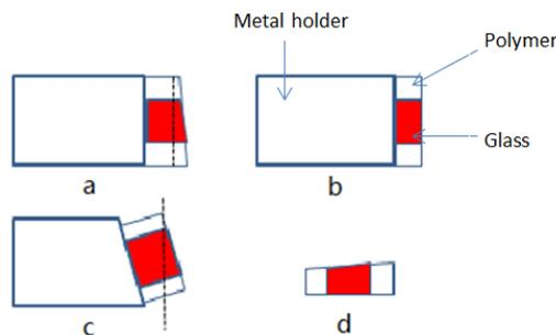
Figure 1 Schematic diagrams showing the prism preparation procedure
