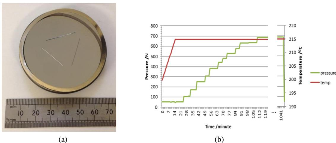
Figure 2 (a) Three  $\text{As}_{40}\text{Se}_{60}$  (at%) fibres surrounded by a  $25\ \mu\text{m}$  thick stainless steel shim placed on a tungsten carbide plate ready for hot pressing. (b) Typical pressing schedule for  $\text{AsSe}$ .
