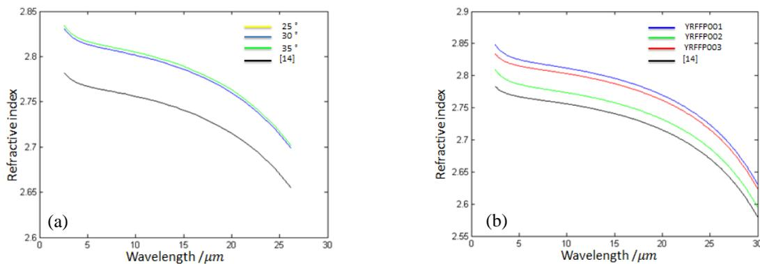
Figure 4 (a) Refractive index data for  $As_{40}Se_{60}$  (at%) fitted by a two-term Sellmeier equation obtained using the Swanepoel method for the sample shown in Figure 4 obtained with different incident angles. (b) Similar results obtained from a set of samples pressed on different occasions. Both plots also present the data from [14] for comparison purposes.
