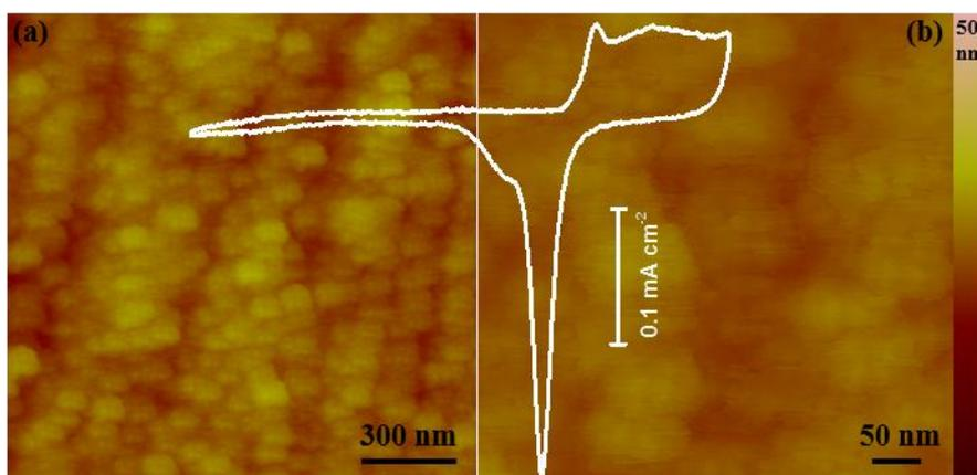
Figure 1. (a) and (b) AFM images of Au Film, and the inset shows a representative CV we obtained for Au-film electrode. The CV was recorded in 0.1M HClO<sub>4</sub> electrolyte saturated with Ar; the potential limits are -0.1 to 1.35V<sub>SCE</sub>, the scan speed was 50 mV/s.
