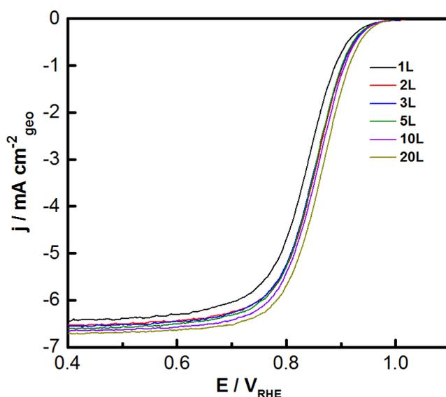
Figure 3. Positive going polarization curves of the PtAu-film electrodes with different amounts of nominal Pt layers; the scan speed was 50 mV/s, the electrolyte  $O_2$  saturated 0.1M  $HClO_4$  solution, and the rotation rate 1600rpm.
