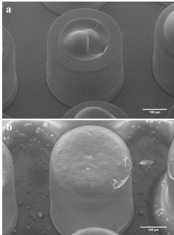
Fig. 2: SEM picture of drug loaded microcontainer: (a) before and (b) after the Eudragit L100<sup>®</sup> coating.
