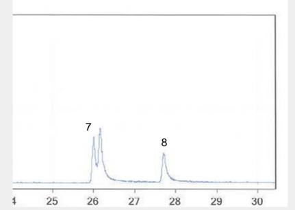
Figure 3. Whisky light chromatogram of  $m/z = 252$  at the top, namely benzo[b]fluoranthene (5) and benzo[a]pyrene (6) and  $m/z = 264$  with benzo[b]fluoranthene D12 (7) and benzo[a]pyrene D12 (8) at the lower part
