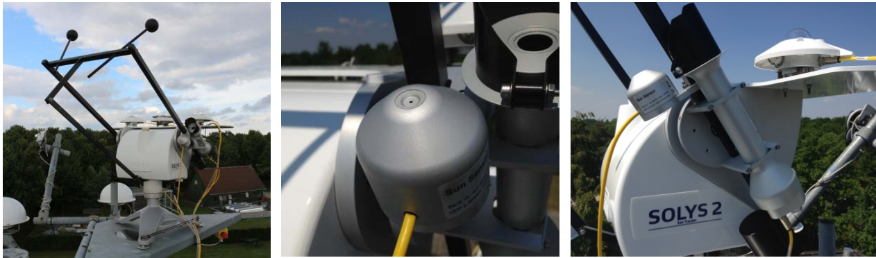
Figure 3: The SOLYS 2 tracker. On the top mounting plate, the solar radiation measurement instruments can be seen. On the left side of the tracker, the solar sensor and the pyrheliometer that measured the shortwave beam normal irradiance can be seen.
