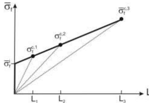
**Figure 3.** Sketch of the relation between fibre stress and debond length according to eq (2) and (5) for traditional pull-out experiments, the dotted slopes indicate the calculations of the *apparent* shear stress, which for this case is *decreasing* with increasing embedded fibre length (termed L)
