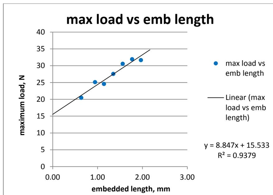
**Figure 6.** Experimental data for steel fibre in epoxy matrix
