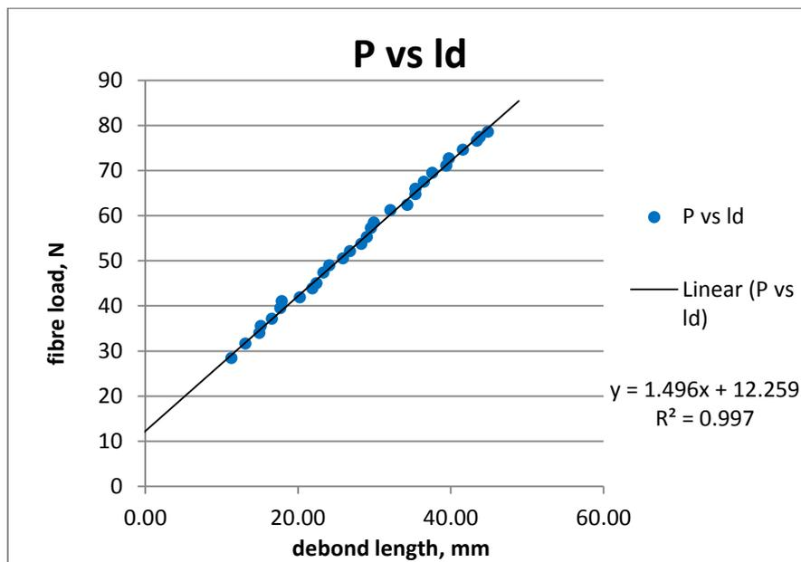
**Figure 4.** Experimental data for steel fibre in polyester
