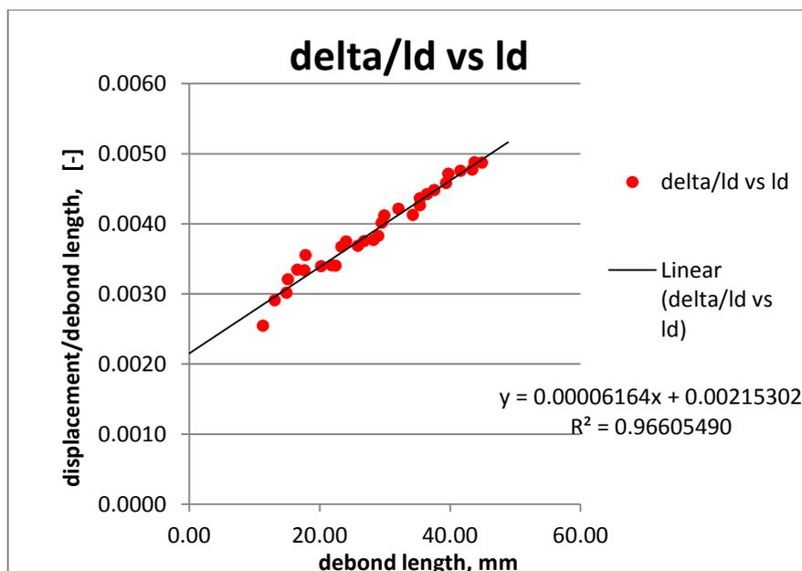
**Figure 5.** Experimental data for steel fibre in polyester
