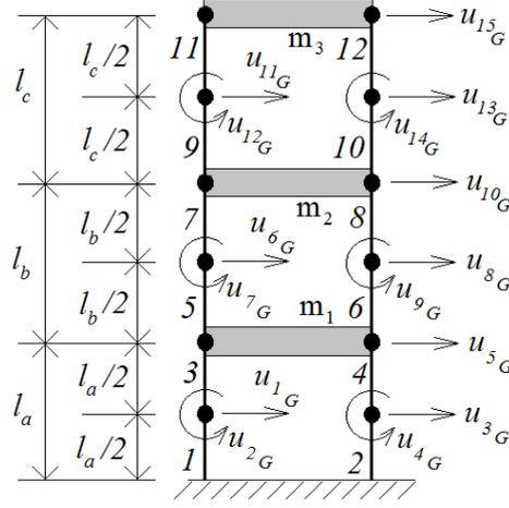
**Fig. 3** Discretized structure
