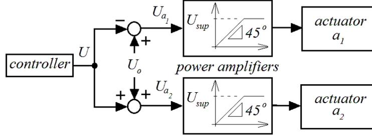
**Fig. 5** Voltage saturation
