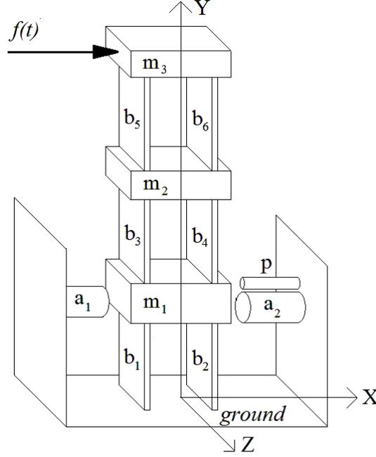
**Fig. 1** Shear frame structure
