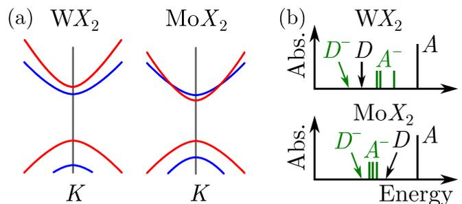
FIG. 3. (a) Schematic band alignment in WX<sub>2</sub> and MoX<sub>2</sub> (*X* = Se/S) around *K*. The color denotes the spin character of the bands, i.e., only a transition with spin conservation can be optical active. (b) Sketch of expected absorption spectra including dark excitations.
