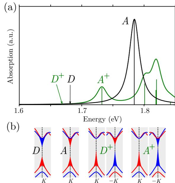
FIG. 2. (a) Optical absorption spectrum of WSe<sub>2</sub> of excitons (black) and positively charged trions (green) near the lowest possible transitions. (b) The contributions of the dark *D* and bright *A* exciton, as well as the dark *D*<sup>+</sup> and *A*<sup>+</sup> trions. For more details, see the caption of Fig. 1.
