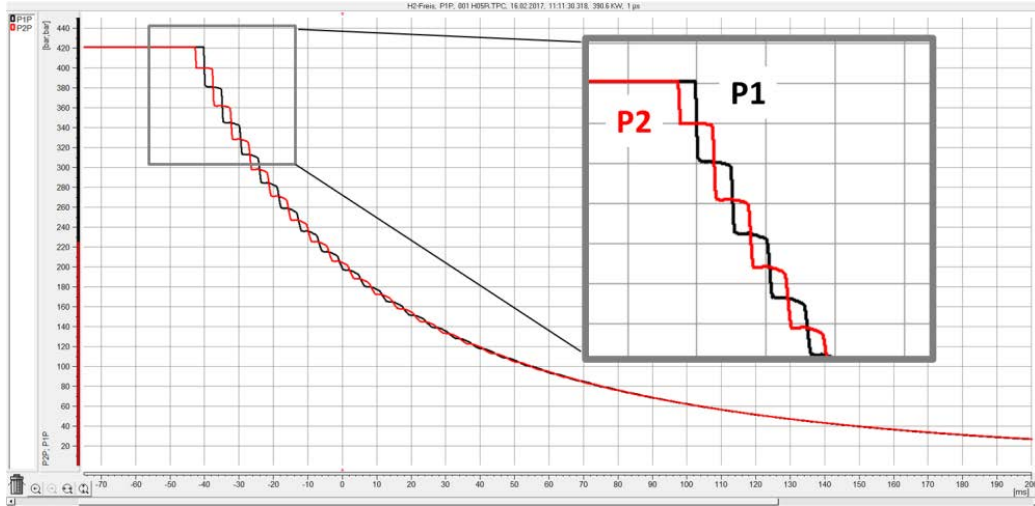
Figure 10: Pressure decay curves inside the high-pressure storage tube for sensor P1 in black color at the upstream end of the tube and sensor P2 in red color at the downstream end of the tube close to the reduction to the release pipe.
