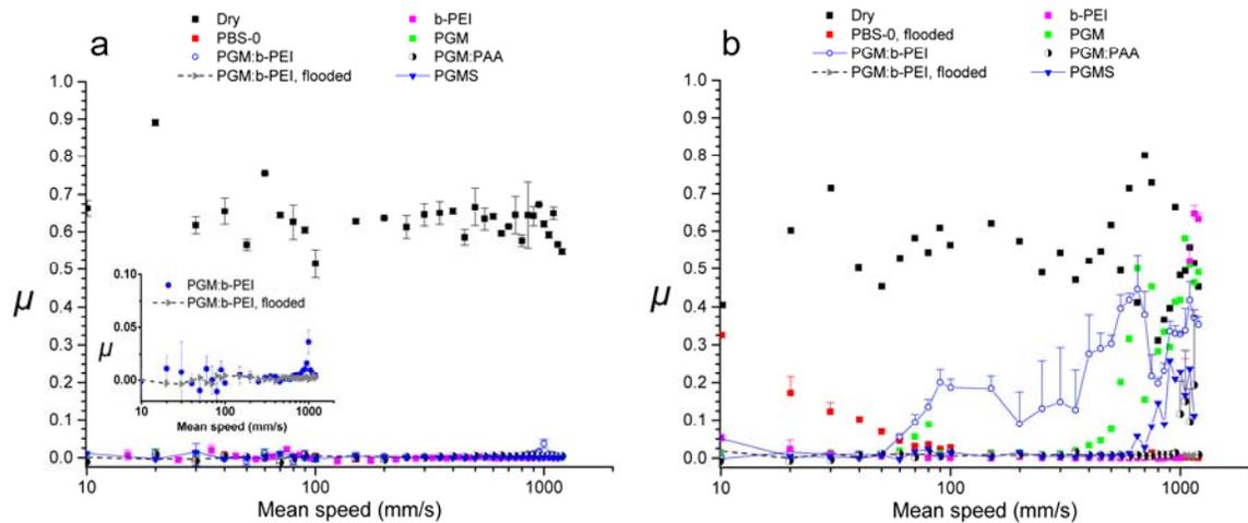
FIG. 5.  $\mu$  vs speed measured with MTM for (a) steel-PDMS and (b) PDMS-PDMS interface lubricated with the mucus samples (load = 5 N, SRR = 10%) For PGM and PGMS, only data points from the first speed sweep are shown due to much higher friction in the second sweep caused by centrifugation depletion. Mucus samples were applied as thin film lubricants, unless ‘flooded’ is stated. Some negative error bars were removed for clarity. The lines connecting the data points are a guide to the eye.
