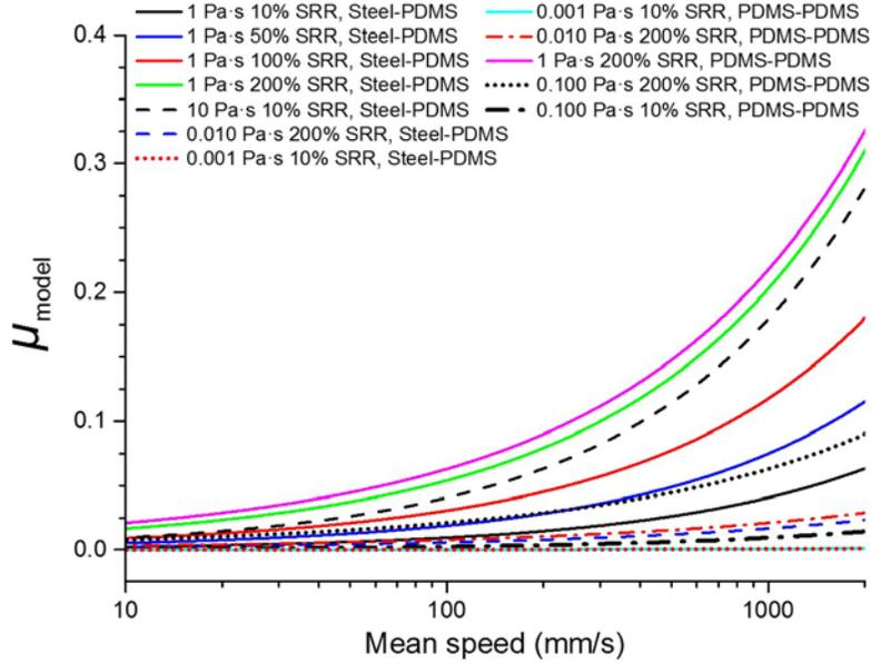
FIG. 3. Friction coefficients ( $\mu$ ) calculated from Equation 2 as a function of the mean speed ( $u$ ), viscosity (in Pa·s) and SRR ratios for steel-PDMS and PDMS-PDMS contacts (5 N load) lubricated by generic Newtonian fluids. The model assumes constant viscosity as in a previous study by de Vicente et al.<sup>37</sup>
