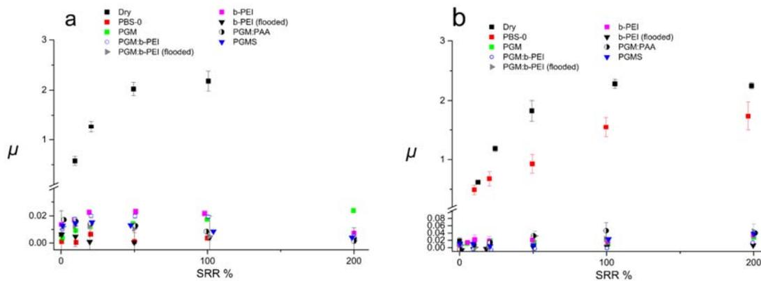
FIG. 7.  $\mu$  vs SRR for (a) steel-PDMS interface and (b) PDMS-PDMS interface lubricated with thin films of mucus samples as characterized with MTM (speed = 20 mm/s, load = 5 N). Friction was too high in the dry contact for the measurements to commence at 200% SRR for steel-PDMS.
