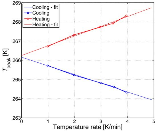
Figure 4: Heat capacity peak temperature,  $T_{\text{peak}}$ , as a function of temperature rates for both heating and cooling. At finite heating and cooling rates extrinsic hysteresis is apparent. However, the intrinsic hysteresis, corresponding to the extrapolated temperature rate 0 K/min, vanishes.
