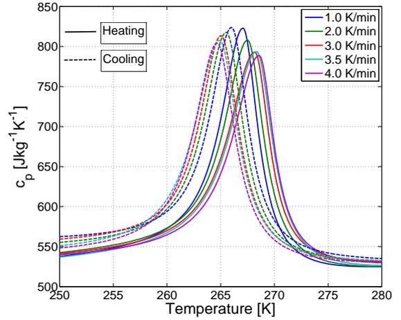
Figure 3: Specific heat as a function of temperature for different temperature rates at 0 T.
