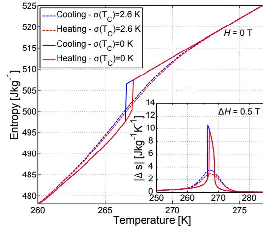
Figure 9: Entropy as function of the temperature, for heating and cooling procedures, and  $H = 0$  T. One may see the vanishing impact of the distribution  $\sigma(T_C)$  on the hysteresis. The inset shows the modelled isothermal entropy change for  $\Delta H = 0.5$  T, during heating and cooling procedures.
