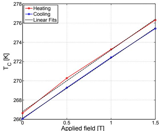
Figure 6: The specific heat peak temperature,  $T_{\text{peak}}$ , as a function of applied magnetic fields for both heating and cooling heat capacity measurements, with  $|\dot{T}| = 1.0$  K/min. The dashed lines are linear fits.
