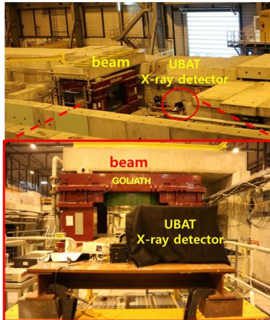
**Figure 5:** Test set up at H4 beam line of CERN. The dark box which includes X-ray detector is placed in front of beam line.
