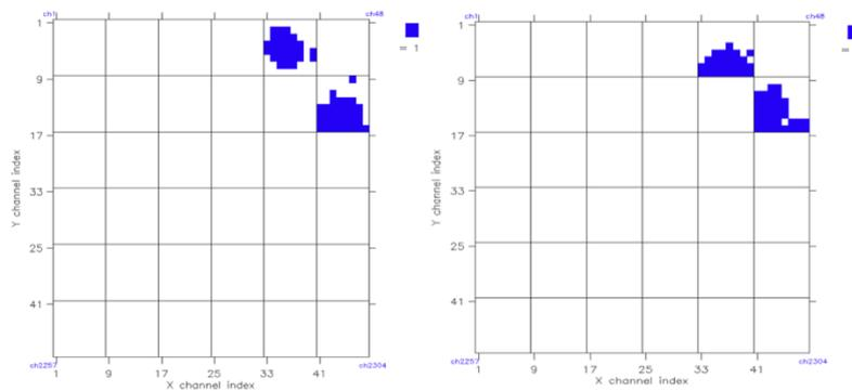
**Figure 6:** Each is one of frames response from beam test. It takes 6msec to take a frame data. UBAT has 6×6 MAPMTs originally but mini UBAT has only 2 MAPMTs. Its locations are (1,5) and (2,6). Blue color is response for any particles and white color is no response.
