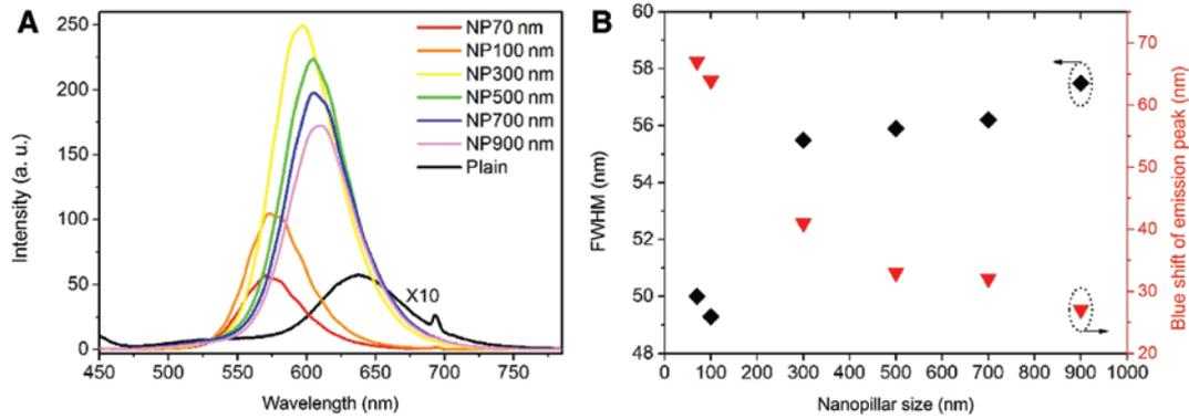
**Figure 2:** (A) PL spectra of different nanopillar samples and plain reference sample. The spectra are obtained under identical measurement conditions and the surface reflection of excitation laser beam has been taken into account. (B) Emission peak wavelength and FWHM of PL spectra as a function of the nanopillar size.
