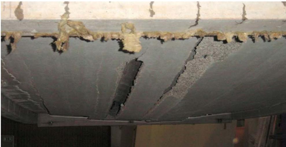
Figure 8. Damages after 25 minutes. Photo K. Hertz.
