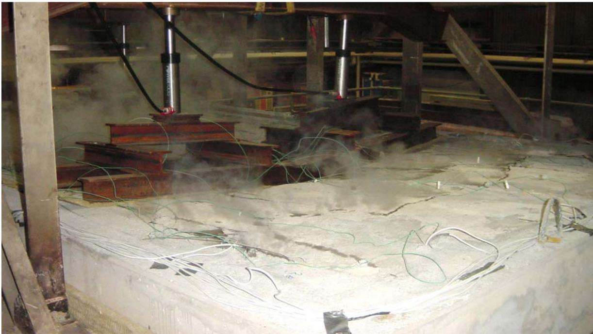
Figure 7. Cracks in top flange after approx. 15 min. Photo K. Hertz.
