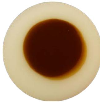
Figure 2. Top view photo of one of the YSZ pellets with LSCF film (S2D). The diameter of the YSZ pellet is 9 mm, and that of the LSCF film is 5 mm. The LSCF thickness is  $495 \pm 5$  nm in the uniform darkest area. The thinner areas are caused by shadow mask drift during deposition.
