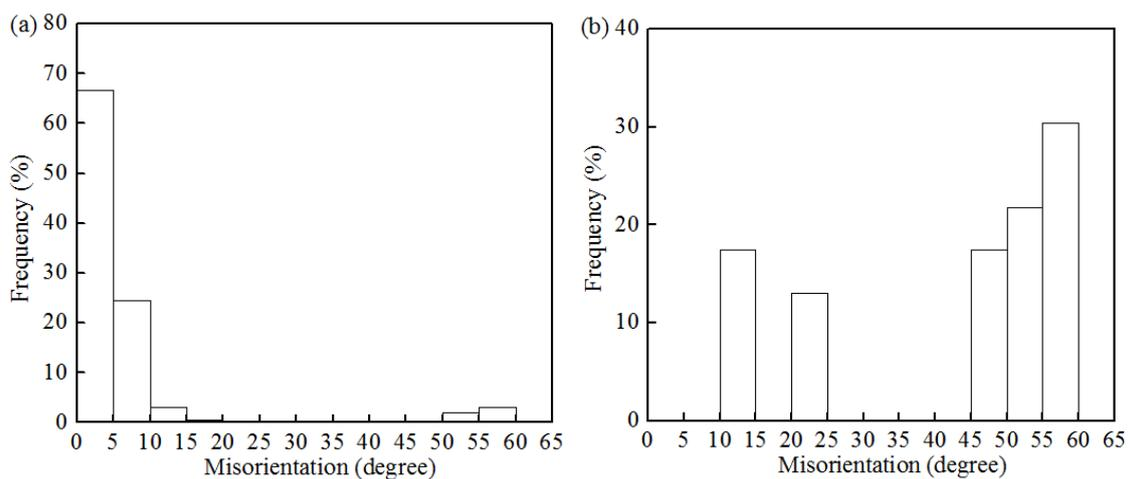
**Figure 3.** Misorientation angle distribution in un-deformed martensite: (a) from EBSD maps, excluding prior austenite grain boundaries; (b) between V1 and other variants (V2-V24) based on the K-S orientation relationship.
