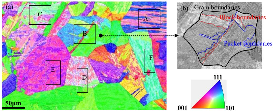
**Figure 2.** EBSD map of the un-deformed as-transformed martensite.
