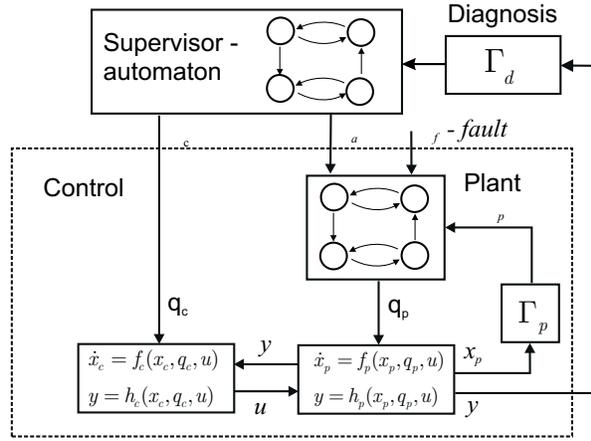
Fig. 1. Fault tolerant control systems are hybrid by nature. The dynamics of the plant is influenced by mode changes  $q_p$ , the controller by  $q_c$ .  $\sigma_f$  denote fault events,  $\sigma_a$  control events. Plant internal events are  $\sigma_p$ .
