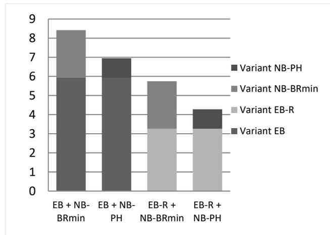
**Figure 3: Four demand variants for end-user heating energy demand (in GWh/a). EB stands for the end-user heating energy demand of the non-renovated building stock, EB-R for the renovated building stock, NB-BRmin for the new buildings built after minimal standard of the building regulation code, and NB-PH for the new buildings built in passive house standard.**
