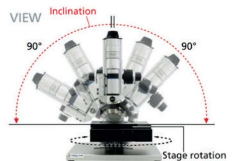
Figure 3. Hirox RH-2000 digital microscope.
