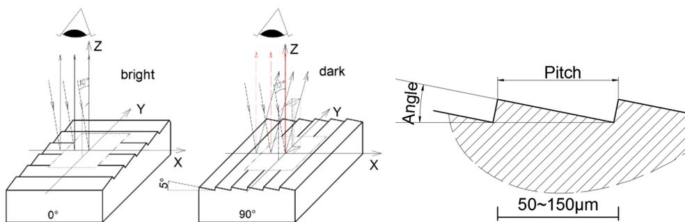
Figure 1. Contrast generation and structure of the surface.
