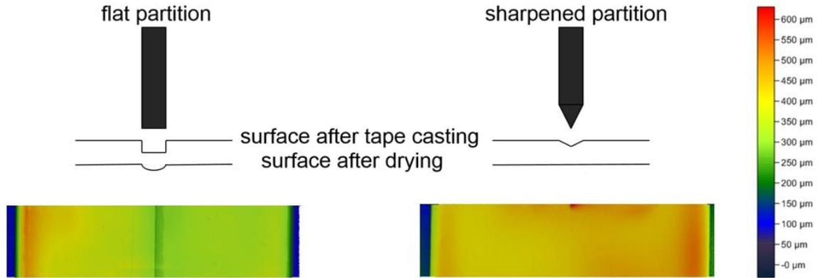
Figure 4. Schematic representation of surfaces of green graded tapes after co-casting using a non-sharpened and sharpened partition and below the pictures of surface topography of green tape samples, which were analysed by means of laser profilometry. The short slit on the sample, cast with the tapered partition, was made by knife in order to later identify the interface region on a completely smooth graded tape. The length of each piece of tape was 20 mm, and the width was 80 mm.
