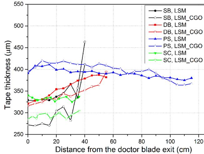
Figure 3. Thickness deviation of tapes, cast with usage of single-blade (SB), double-blade (DB), single blade and pump system (PS), single-blade and a program of casting speed change (SC). The estimated error in tape thickness measurement is 15  $\mu\text{m}$ .
