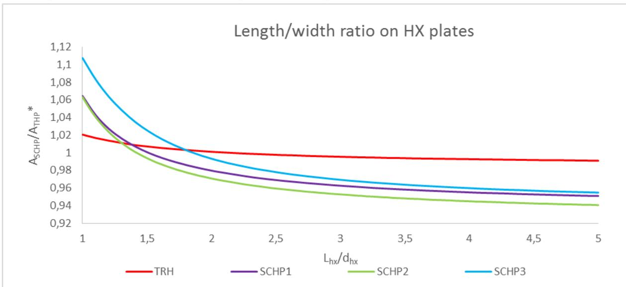
Figure 4: Relative area of plate heat exchangers on high pressure side of the heat pump as a function of the length/width ratio of the plates. Length/width ratio of plates is the same in both heat exchangers. The red curve corresponds to the traditional heat pump. SCHP1-3 corresponds to different plate dimensions for the split condenser heat pump.
