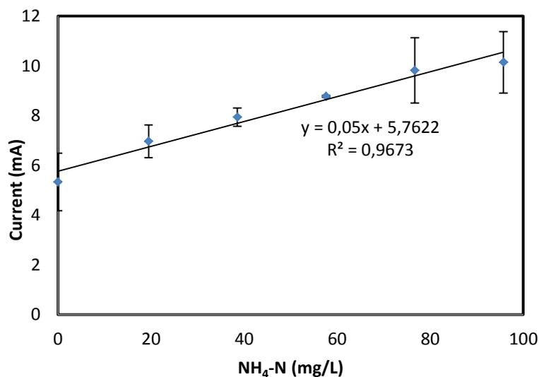
Figure 3. Linear relationship between current and ammonia levels at external voltage-1.8V and solution pH-6.
