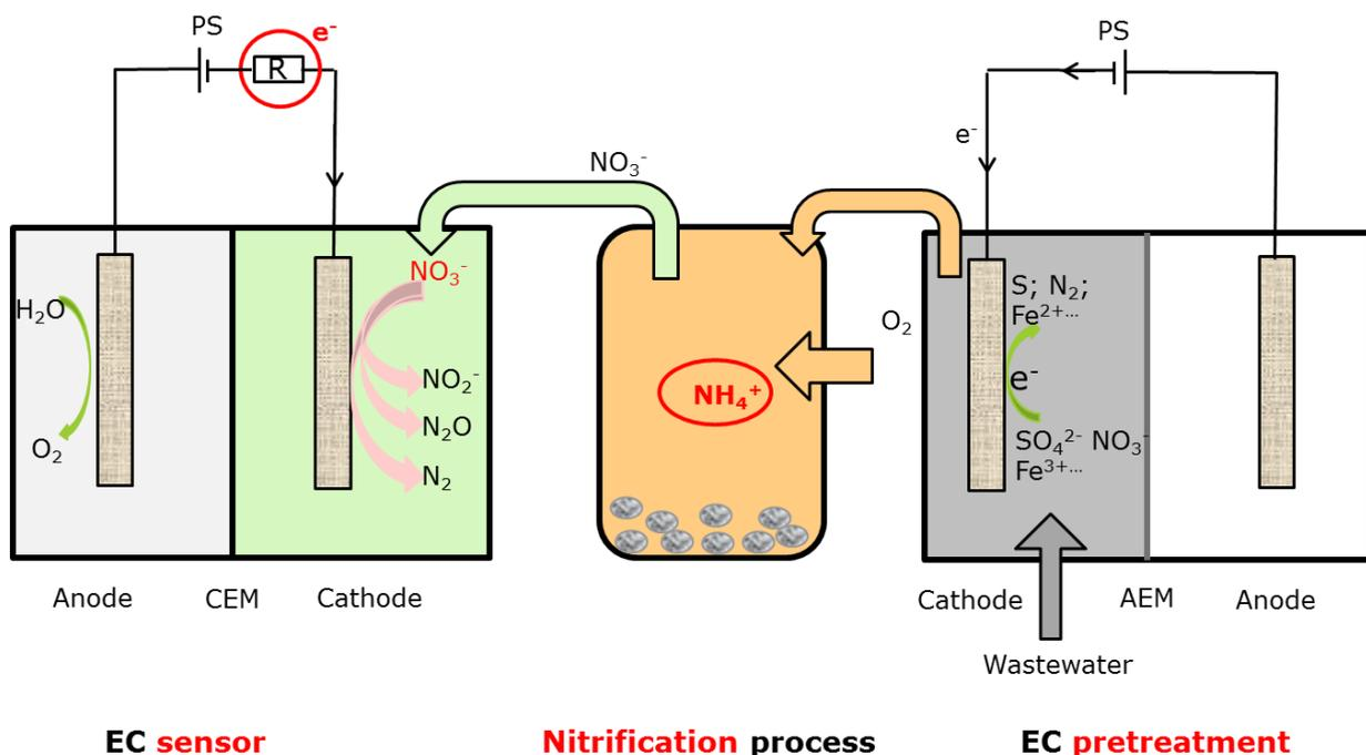
Figure 1. Schematic diagram of EC sensor, nitrification reactor and EC pretreatment.
