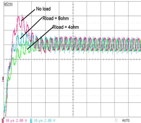
Figure 14 Measured step response of prototype – 2V/div and 10µs/div
