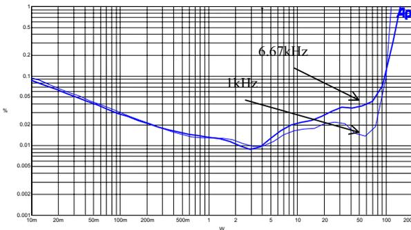
Figure 16 THD+N ratio of prototype amplifier with 4Ω load at 1kHz and 6.67kHz, 80kHz measurement bandwidth
