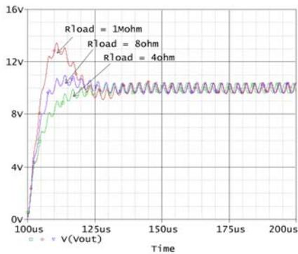
Figure 12 Simulated step responses of prototype amplifier design
