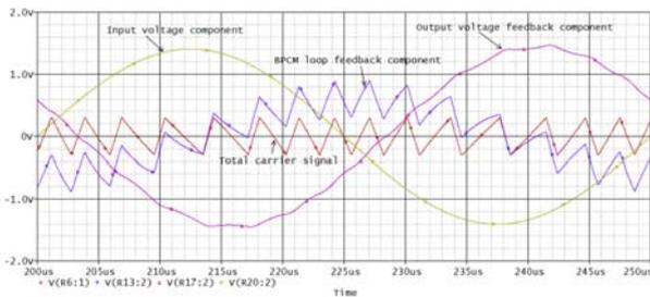
Figure 8 Simulated, optimized carrier signal and its subcomponents in prototype amplifier design. Amplifier producing 20kHz sinewave output at  $M=0.75$  with  $8\Omega$  load.
