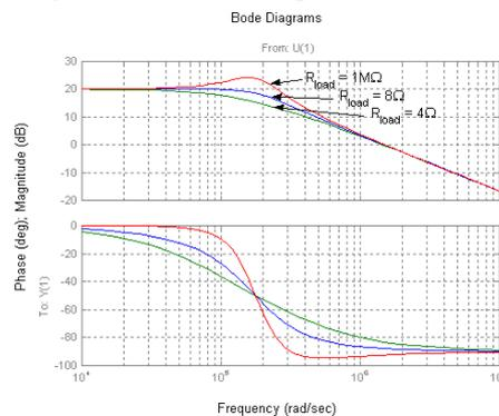
Figure 10 Closed-loop Bode plots of prototype amplifier design
