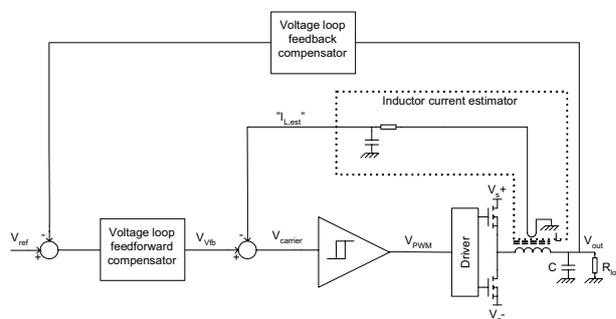
Figure 1 Basic structure of the proposed control scheme
