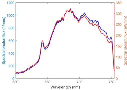
**Figure 1.** Spectra of the NV-centre emission: absolute photon flux per wavelength  $N_{\text{ph},\lambda}(\lambda)$  (blue line) and absolute radiant flux per wavelength  $\Phi_{\lambda}(\lambda)$  (red line).
