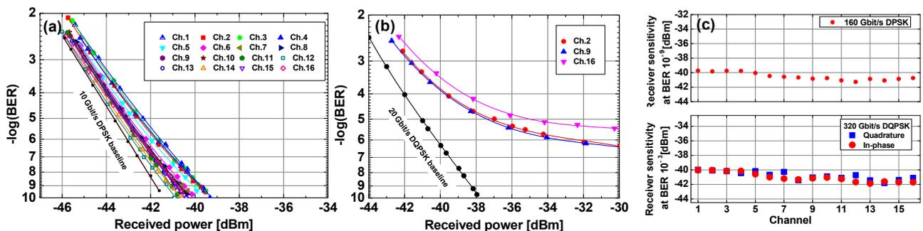
Fig. 3. Experimental results. (a) BER performance of all 16 demultiplexed 10-Gbit/s DPSK channels, (b) BER performance for selected demultiplexed DQPSK channels, (c) receiver sensitivities at  $\text{BER} = 10^{-9}$  of all demultiplexed DPSK channels, and receiver sensitivities at  $\text{BER} = 10^{-3}$  of all DQPSK channels.
