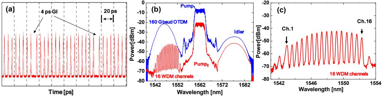
Fig. 2. Results of OTDM to WDM conversion. (a) 160 Gbaud OTDM signal waveform, (b) optical spectrum after the first (blue curve) and second (red curve) FWM process, (c) spectrum of the 16 obtained WDM channels.
