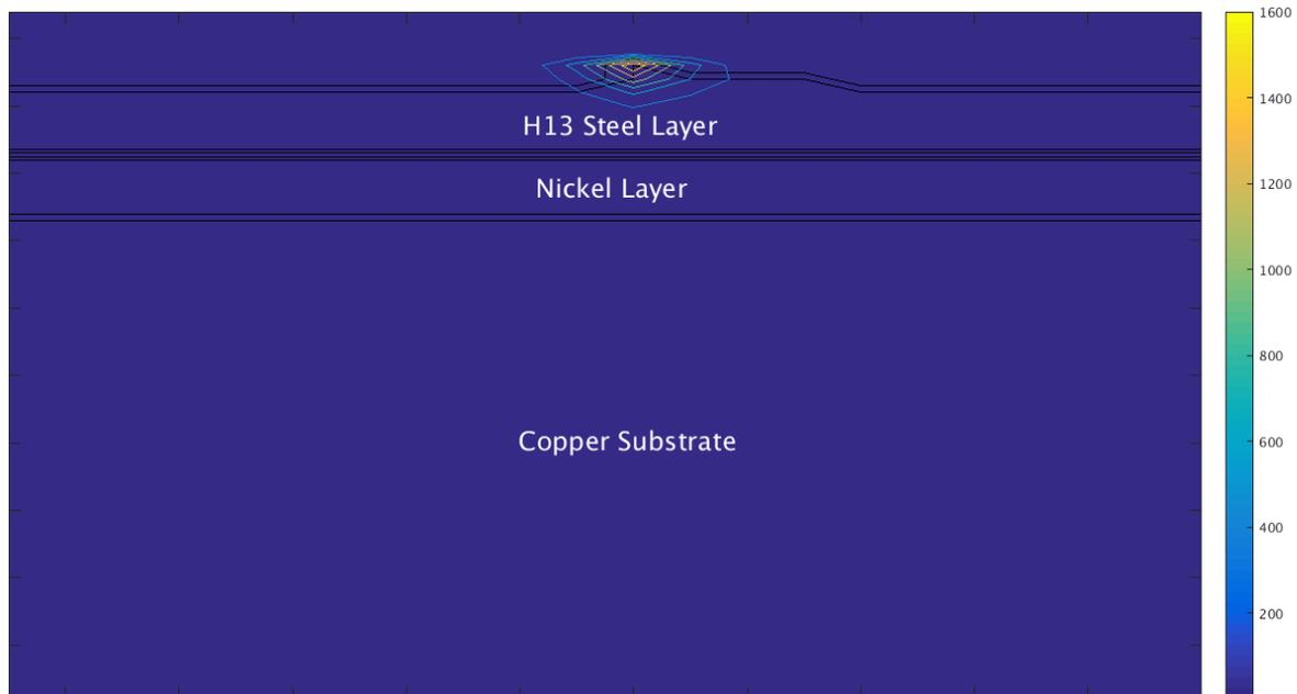
**Figure 4 Temperature distribution in transverse cross-section of the sample during SLM of third layer of H13 steel (super-imposed on the material distribution)**
