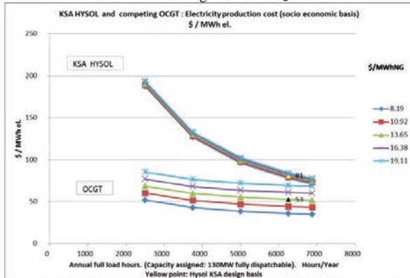
Figure 1 Electricity production costs for Open Cycle Gas Turbine (OCGT) and KSA HYSOL configuration, as function of load factor and NG price. Assumed: CO<sub>2</sub> costs = 0\$/tonCO<sub>2</sub>, R=4%p.a., Lifetime=25years. Unit: \$/MWh el.
