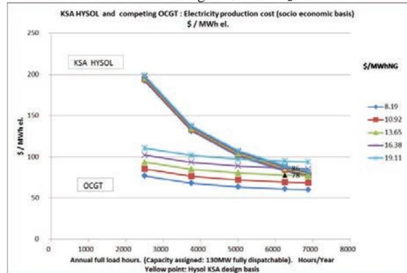
Figure 2 Electricity production costs for Open Cycle Gas Turbine (OCGT) and KSA HYSOL configuration, as function of load factor and NG price. Assumed: CO<sub>2</sub> costs = 40\$/tonCO<sub>2</sub>, R=4%p.a., Lifetime=25years. Unit: \$/MWh el.
