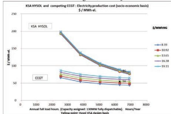
Figure 4 Electricity production costs for Combined Cycle Gas Turbine (CCGT) and KSA HYSOL configuration, as function of load factor and NG price. Assumed: CO<sub>2</sub> costs = 40\$/tonCO<sub>2</sub>, R=4%p.a., Lifetime=25years. Unit: \$/MWh el.
