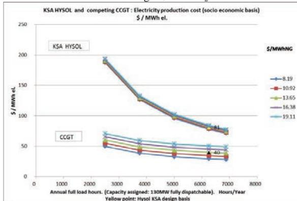
Figure 3 Electricity production costs for Combined Cycle Gas Turbine (CCGT) and KSA HYSOL configuration, as function of load factor and NG price. Assumed: CO<sub>2</sub> costs = 0\$/tonCO<sub>2</sub>, R=4%p.a., Lifetime=25years. Unit: \$/MWh el.
