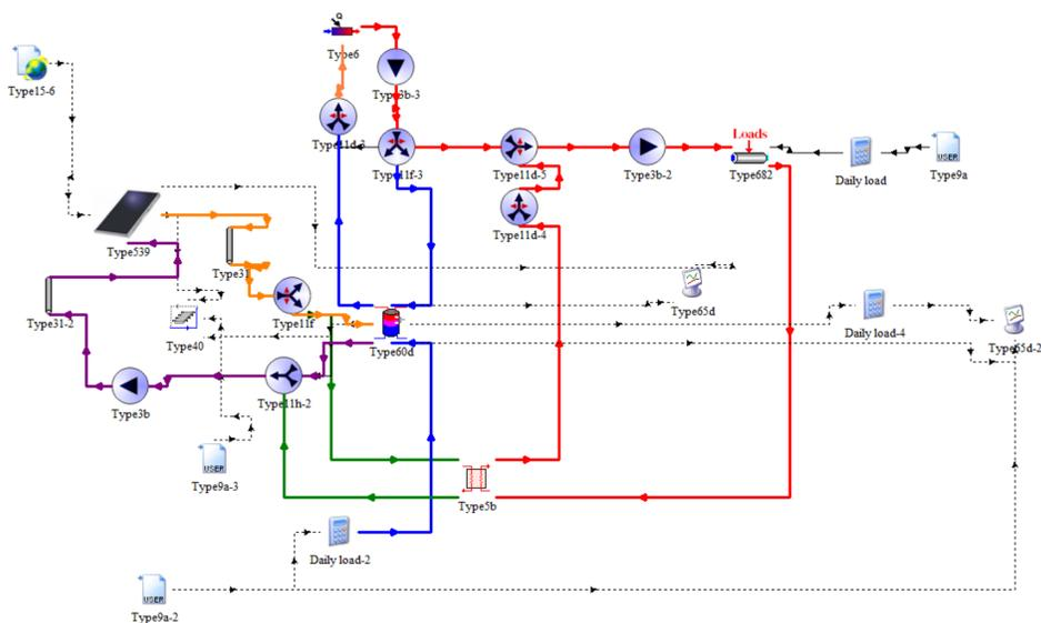
TRNSYS model of the solar collector system
