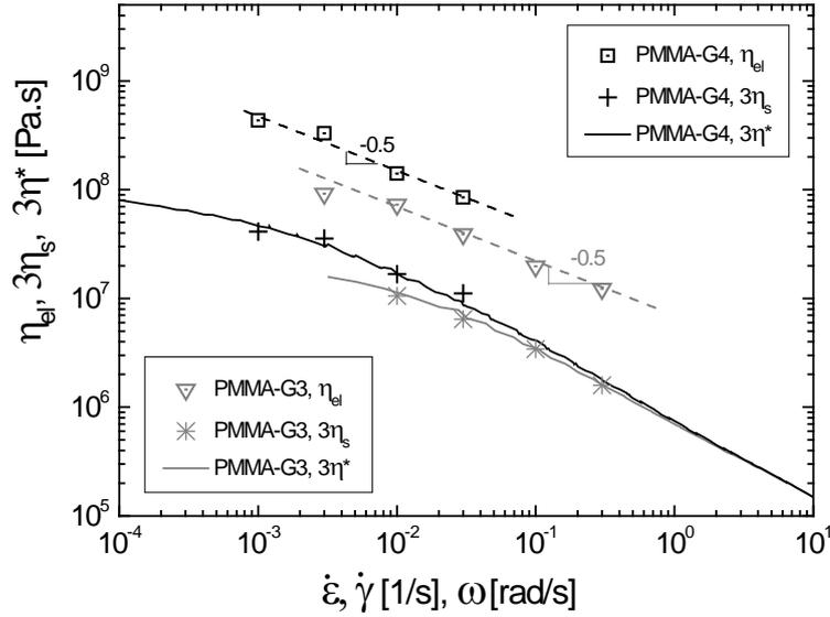
**Figure 7:** Steady-state data on extensional viscosity (open symbols), shear viscosity (crosses and stars) and dynamic complex viscosity (solid lines, multiplied by the Trouton ratio 3) plotted against Hencky strain rate, shear rate and oscillatory frequency, respectively, on the same axis. Data are shown for G3 (gray) and G4 (black). The dashed lines through the extensional data have a slope of -0.5.
