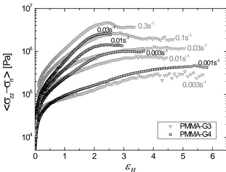
**Figure 6:** Net tensile stress for G3 (gray) and G4 (black) versus Hencky strain for different values of the imposed Hencky strain rate, at 180°C.
