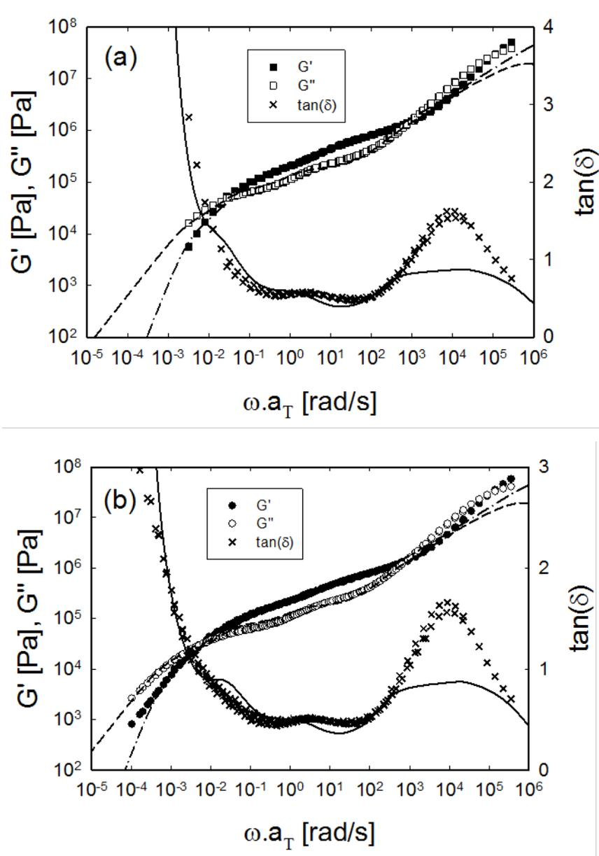
**Figure 2:** Linear viscoelastic master curves from van Ruymbeke et al. [19], depicting  $G'$  (closed circles),  $G''$  (open circles) and  $\tan(\delta)$  (crosses) versus shifted frequency ( $\omega \cdot a_T$ ) at a reference temperature  $T_{\text{ref}}=180^\circ\text{C}$  for G3 (a) and G4 (b). For both graphs, black lines are predictions from BoB model ( $G'$ , dash-dotted line;  $G''$ , dashed line;  $\tan(\delta)$ , solid line).
