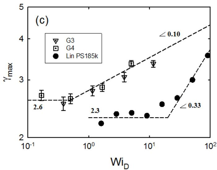
**Figure 5:** (a) Ratio of the stress growth coefficient to the respective LVE value at different stretch rate for G3 (gray) and G4 (black) (b) Normalized peak viscosity and (c) peak strain at the maximum viscosity as functions of the Weissenberg number based on the inverse terminal  $G'G''$  crossover (see text). In (b) and (c) we show for comparison data with linear polystyrene LinPS185k, whereas the lines are drawn to guide the eye (see text).
