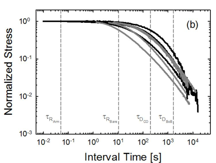
**Figure 9:** Data of Figure 8 normalized by the respective values of shear stress or stress growth coefficient when shear or extensional flow was stopped (see text). Characteristic times are reported for reference as in figure 8.
