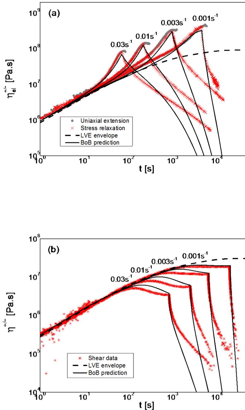
**Figure 4:** Respective data of Figure 3 for the transient response of G4 in uniaxial extension (a) and simple shear (b). The same temperature of 180°C, rates and symbols are used, but different colors (here growth-relaxation cycle is depicted by red). Black solid lines are predictions from BoB model.
