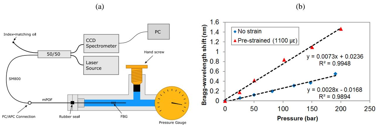
Figure 3. (a) Schematic diagram of the setup used to investigate the pressure response of the FBG. (b) Pressure response of the FBG without pre-strain and an applied pre-strain of  $1100 \mu\epsilon$ . A clear increase in the sensitivity is observed.
