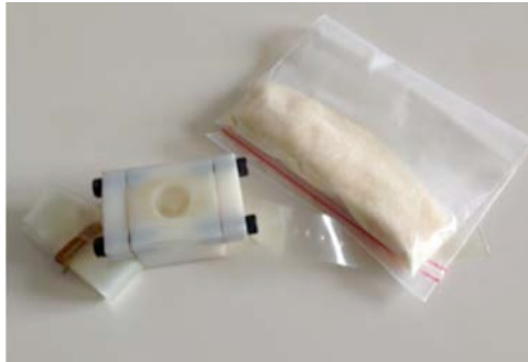
Figure 4: Skin model: gelatin powder, polyurethane membrane and polymer cube.
