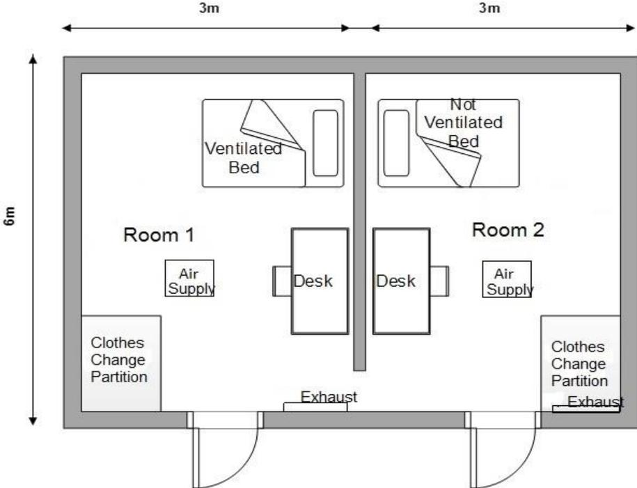
Figure 2 Layout of the experimental set up
