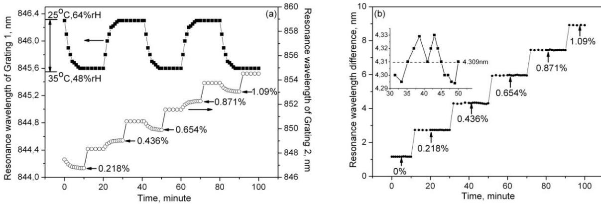
Figure 5. (a) Resonance wavelength of FBG1 and 2 for a temperature alternating between 25 and 35°C (humidity 64 and 38 %rH) every 20 min. while the strain applied to FBG2 alone was increased every 20 min. starting after 10 min. (b) Difference in resonance wavelength of FBG2 and 1. Inset: zoom from 31 to 50 min (adopted from [10]).
