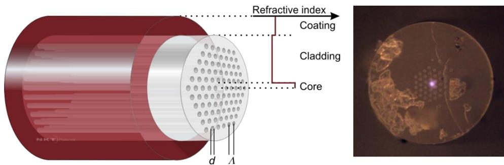
Figure 1. Left: mPOF hole structure with pitch  $\Lambda$  and hole diameter  $d$ , providing a lower average refractive index in the cladding than in the solid core. Right: Visible light being guided in a 3-ring mPOF fabricated at DTU.
