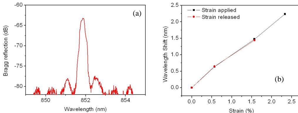
Figure 3. (a) Spectrum of the TOPAS mPOF FBG at  $105^\circ\text{C}$  and no strain applied. (b) Strain response of the TOPAS mPOF FBG at  $105^\circ\text{C}$ . 20 minutes were allowed to reach the equilibrium every time.
